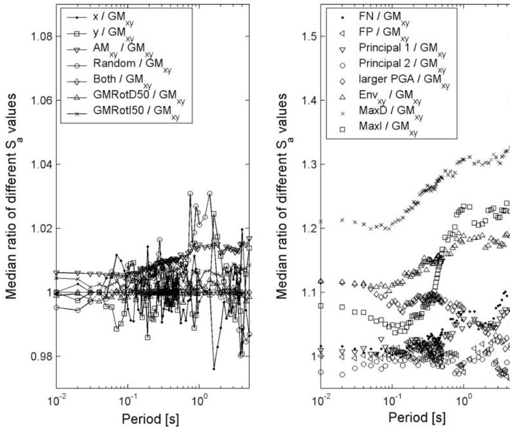
Figure 5. Median ratios of horizontal spectral ordinates for different definitions of the horizontal components of ground motion with the geometric mean of arbitrarily orientated components as reference measure. Note that the y axis of the right-hand panel covers a range of values five times greater than that of the left-hand panel.
