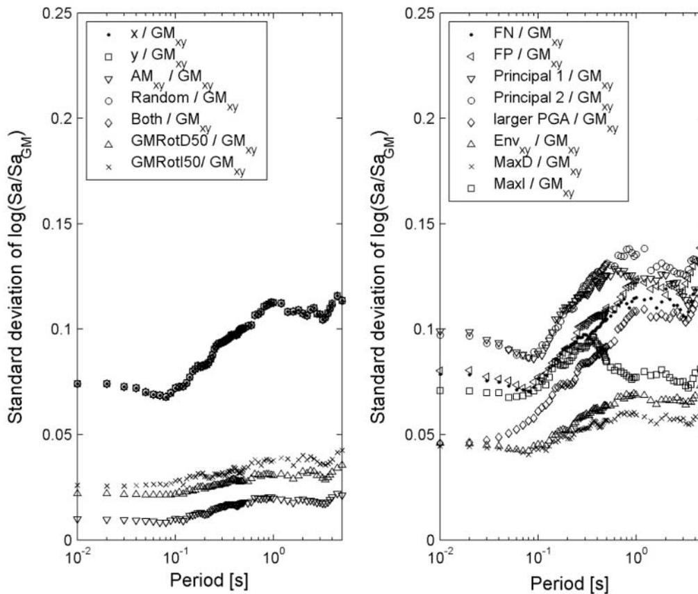
Figure 6. Standard deviation of logarithmic ratios of horizontal spectral ordinates for different definitions of the horizontal components of ground motion with the geometric mean of arbitrarily orientated components as reference measure.
