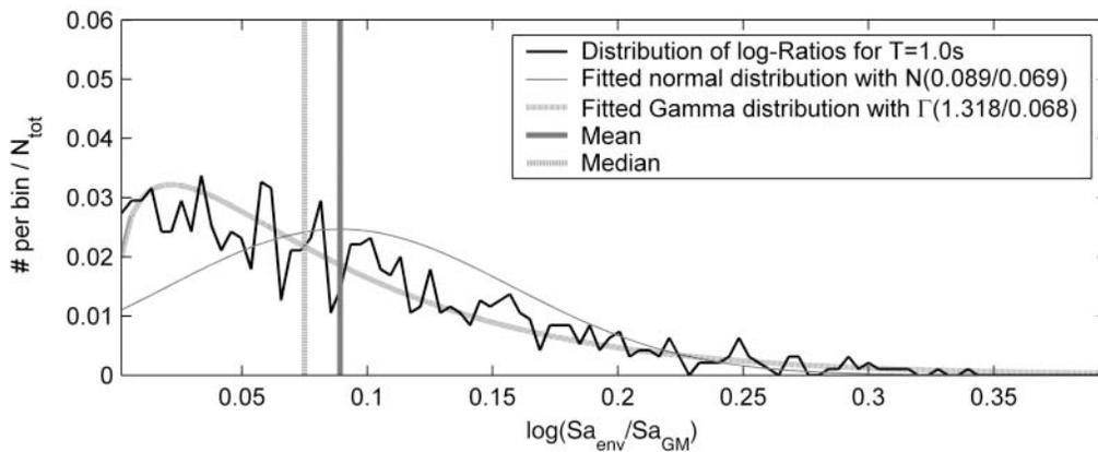
Figure 3. Fitted normal and Gamma distribution to  $\log(Sa_{env}/Sa_{GM_{xy}})$ .
