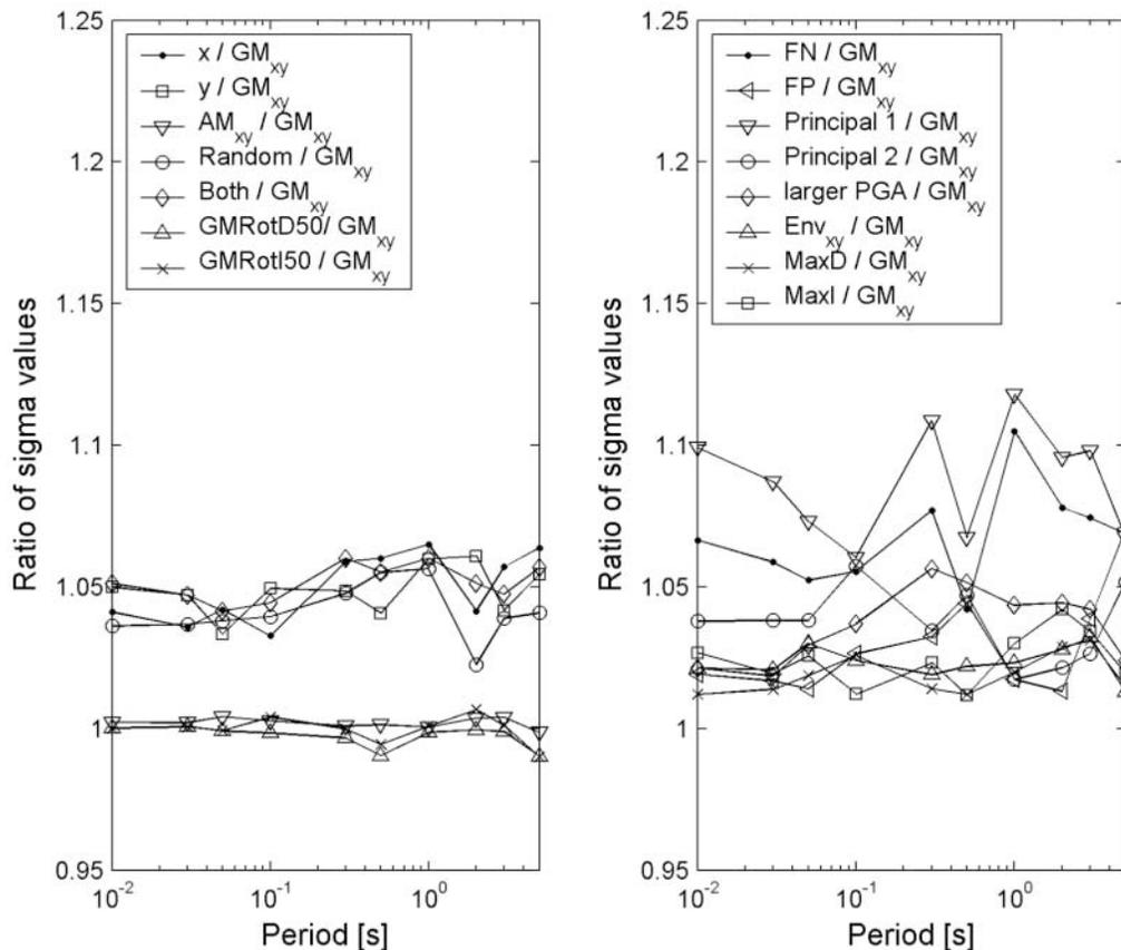
Figure 7. Sigmas obtained from regression analysis for different definitions of the horizontal components of ground motion with the geometric mean of arbitrarily orientated components as reference measure.
