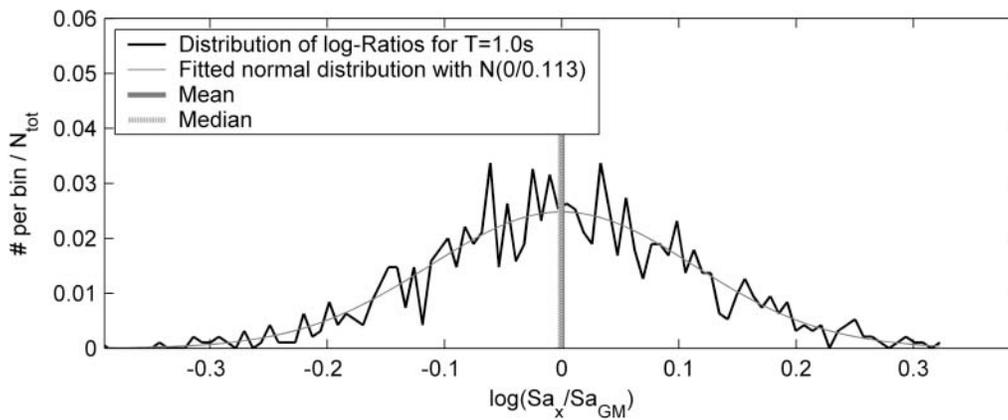
Figure 2. Fitted normal distribution to  $\log(Sa_x/Sa_{GM_{xy}})$ .
